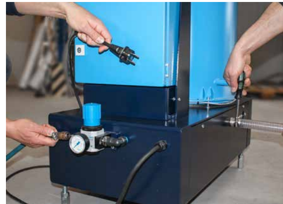
Connections compressed air, electric power and feeding line
